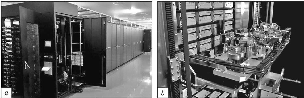
Fig. 4.7. Everspan system full configuration (a), everspan-loading robot (b) [93]
