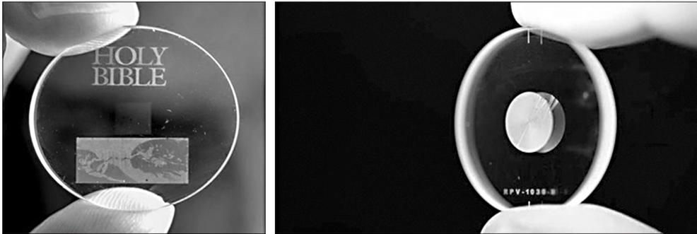
Fig. 5.18. Appearance of fused silica media for long-term storage [172]
